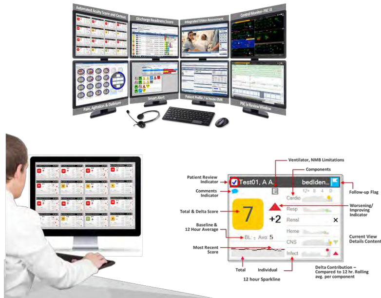
Figure 2: Philips eICU uses AI to Automatically Identify Patients at Risk (Ref. 20)
